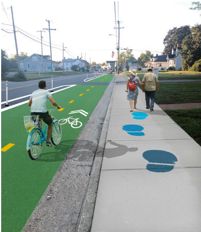
Proposed Condition: Kilmarnock Main Street with dual direction separated bike lanes. 6' sidewalk, 10' bike lane corridor, 2' striped buffer.
