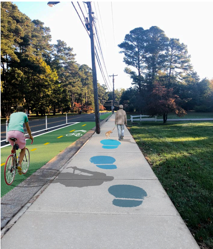
Proposed Condition: Irvington Road with dual direction separated bike lanes. 6' sidewalk, 10' bike lane corridor, 2' striped buffer.
