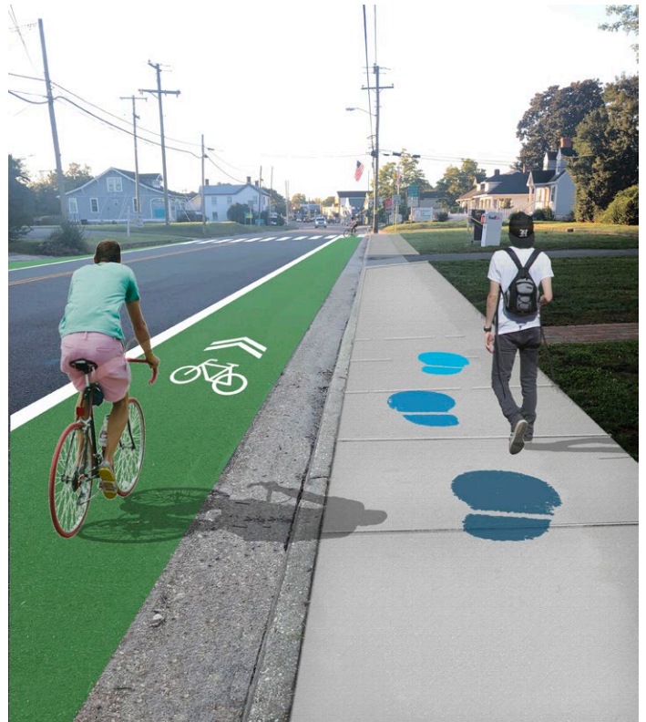
Proposed Condition: Kilmarnock Main Street with single lanes on both sides. 6' sidewalk, two 5' bike lanes on both sides of street.
