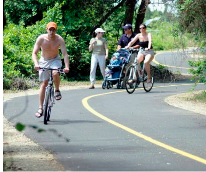
Center stripe for safety (high-traffic areas)
